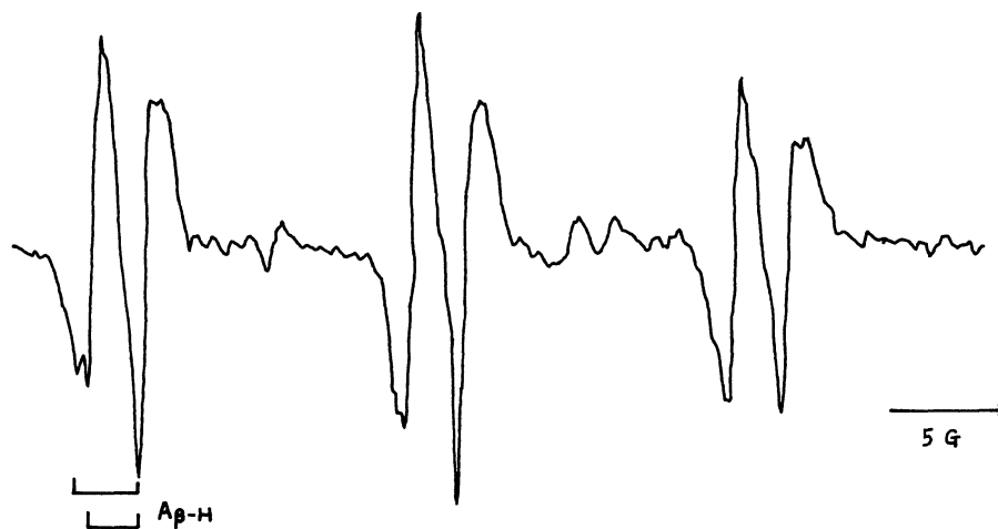
Figure 3. The esr spectrum obtained from r.f. discharge reaction of benzene in the presence of PBN placed in a connecting glass tube between cold trap and discharge reactor.
